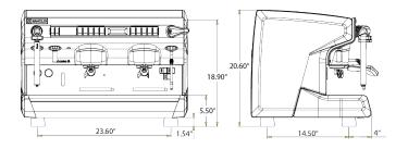
PLEASE NOTE: Power can be installed under or above counter. Please allow 3-4" of space for the plug, especially when placing power above the counter and behind the machine.
